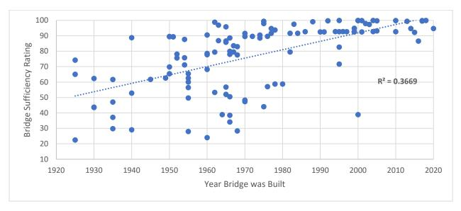
Figure 29: Bridge Sufficiency Rating vs Year Bridge was Built
